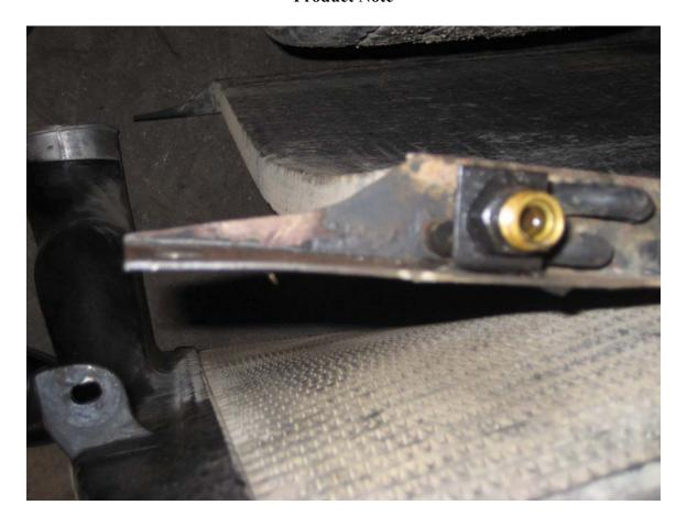
Check the condenser bottom bracket as compared to the unit removed from the truck. If the removed unit looks like the unit shown in the above illustration, proceed to check the truck for hood brace clearance with the hood closed and the old unit bolted in position. If required cut and notch the replacement bracket accordingly.
